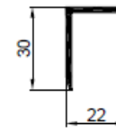
Aluminium spacer profile
